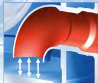
Low inlet into the feed pipe – to prevent steam from entering
